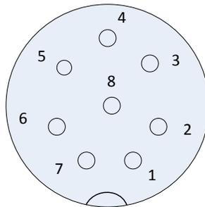
Switchcraft EN3 Connector, Female, 8 Pin Solder Side View
