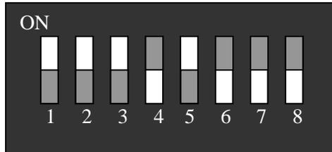
The above diagram shows the default switch settings. Note the darker rectangle is the active side of the switch.
