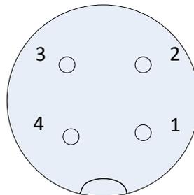
Switchcraft EN3 Connector, Male, 4 Pin Solder Side
