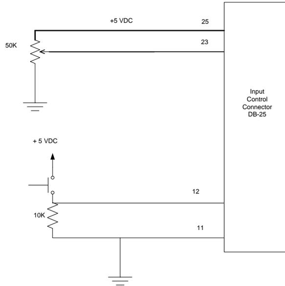
Example of Potentiometer wiring and Push Button wiring above.
