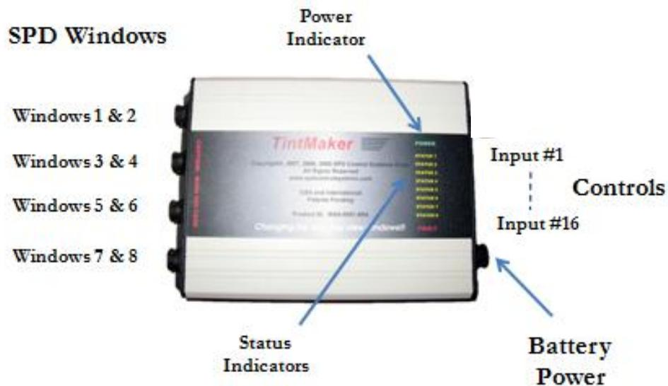
Figure 1.0 - Basic Wiring Connections of the TintMaker/Aftermarket
