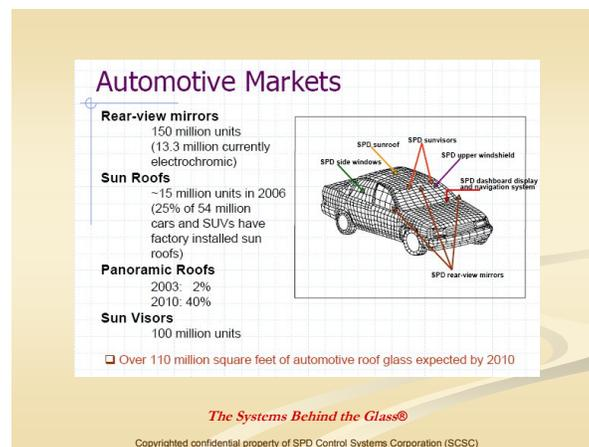
Besides the obvious aesthetic value of SPD windows there is a substantial energy efficiency gain by blocking solar energy. This allows for a less powerful air conditioning unit and reduced air conditioning operation resulting in up to a 10% increase in miles per gallon according to government estimates.
