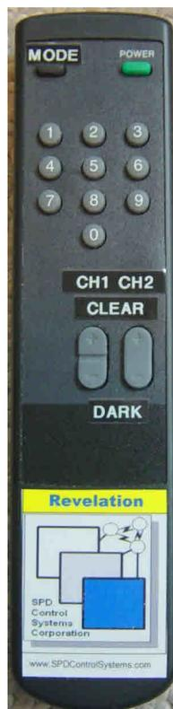
**Figure 5 - Infrared Remote Control**
