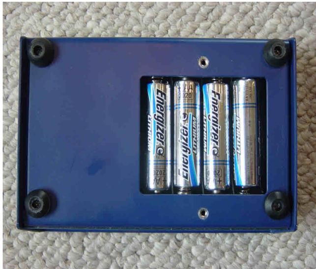
**Figure 3 - Bottom of Demo Unit, Battery Compartment**
